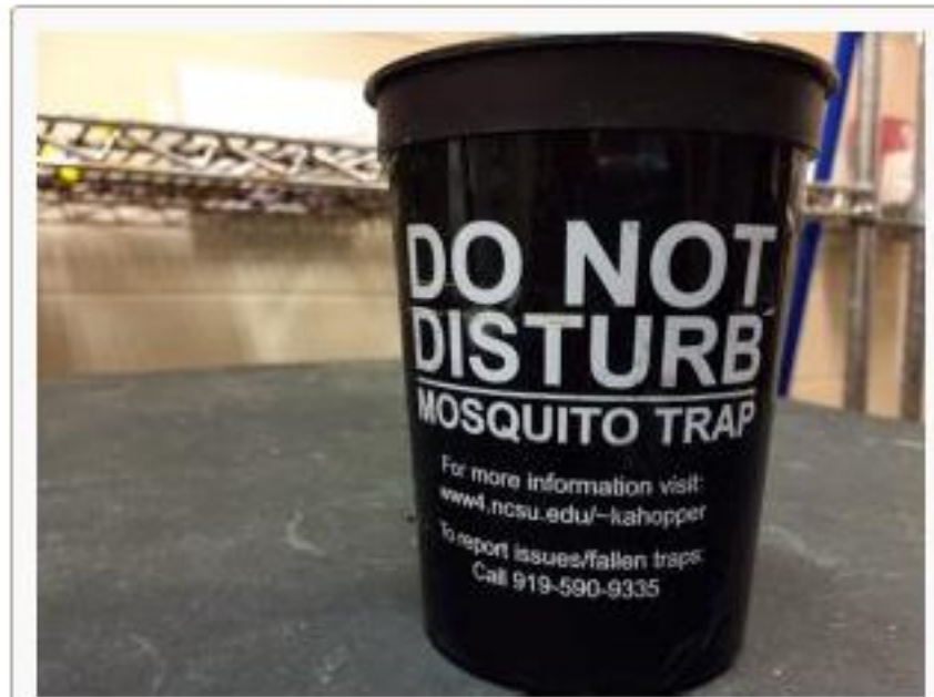
For capturing Aedes mosquito eggs in the wild, plastic stadium cups are the traps of choice. Photo: Catherine Clabby
